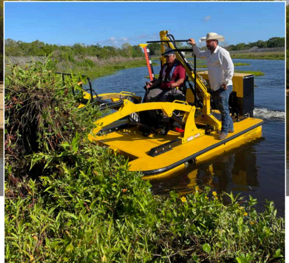
This Brevard County employee is being trained on the newest aquatic vegetation harvesting workboat (shown here removing unwanted aquatic vegetation from a stormwater pond), propelled by its powerful single engine, twin independent outboards. Photo: Brevard County Natural Resources Management Department
