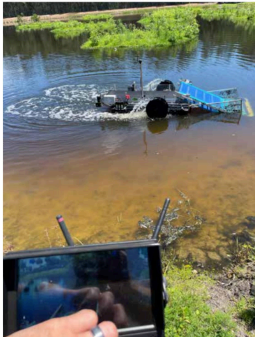
A small, battery-operated, remote-controlled mini harvester patrols this stormwater pond in Brevard County for any unwanted vegetation and debris. Its compact design and ease of use is the perfect addition in a pond management toolkit for tighter, hard to reach areas and small waterbodies. Photo: Brevard County Natural Resources Management Department
