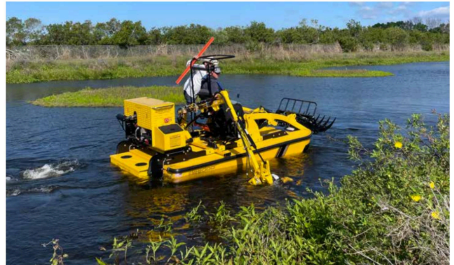
This highly effective vegetation harvesting workboat is equipped with a side cutter bar, deployed here, continuously slicing through emergent vegetation under the water's surface as it hugs the perimeter of the stormwater pond. The vegetation then floats on the surface and, driven by the breeze, gathers to be subsequently collected with the front rake attachment. Photo: Brevard County Natural Resources Management Department
